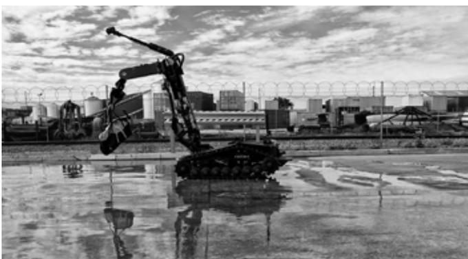
With two independently operated arms (one for the claw and one for disruptors), the robot can easily pick up large items and disrupt them in a safe area. ICOR designed the robot for Large Vehicle Borne Improvised
