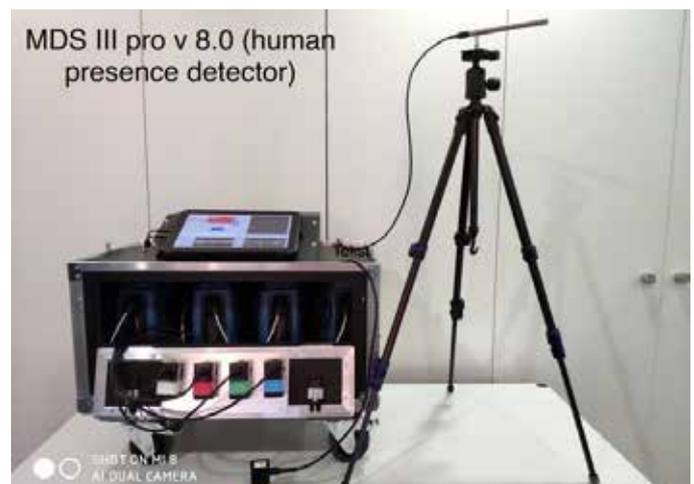
The MDS collects the movements with seismic sensors and analyses the data using an advanced signal processing algorithm.
